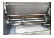
The **DHS** (dynamic hydraulic system) extends the shelf life of your products through lower heat generation in the machine. The **hygiene hydraulic cylinder** makes it impossible for oil to enter into the cutting chamber and contaminate products.
