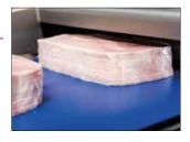
Use the slicer for stacking your products: up to 50 mm high stacks and 300 cuts per minute are possible.
