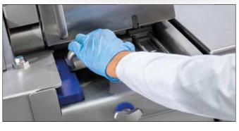
The blade slider prevents stopping of the blade to ensure an **extremely short product loading time - minimising dead time**.
