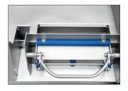
The automatic pre-pressing system (AVS) allow optimum precision shaping of the cubes or strips from the start. It also serves to optimise cycle times through, for example, faster movements in unfilled chamber sections.
