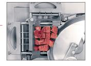
Different cube sizes are possible due to various gridsets. The smallest cube size is 4 mm.
