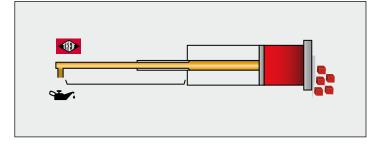
The **hygiene cylinder** (supplied as standard) makes product contamination with hydraulic oil a technical impossibility. No oil can enter the cutting chamber.
