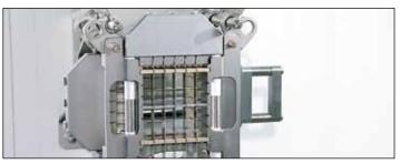
Keep track of things: the special wall bracket is designed for **clean and safe** storage of the gridsets which are currently not in use.
