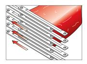
The unique dual-stroke, two-part grid system facilitates precise dicing and strip cutting of the most delicate products by providing twice the normal cutting length at reduced cutting pressure.
