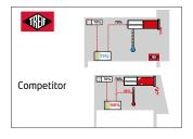
As a result of the DHS (Dynamic Hydraulic System), the cut products stay fresh longer (the machine generates less heat, so there is less of a chance for bacteria to form).
